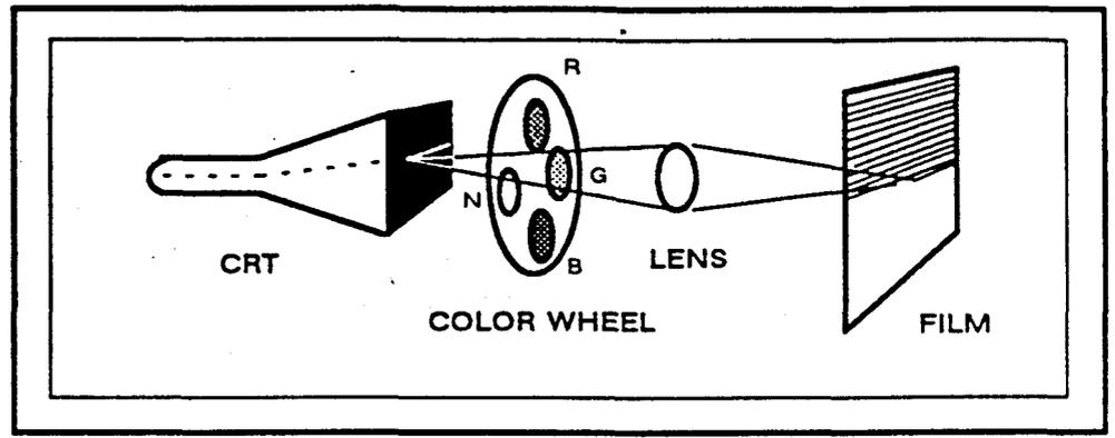
Figure 5-2. SlideWriter Imaging Process
