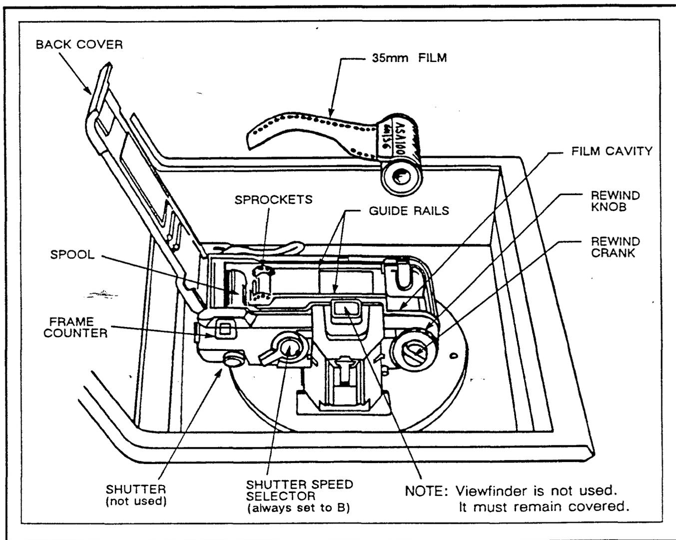
Figure 3-2. Major Components of the Pentax A3000 35mm Camera Back
