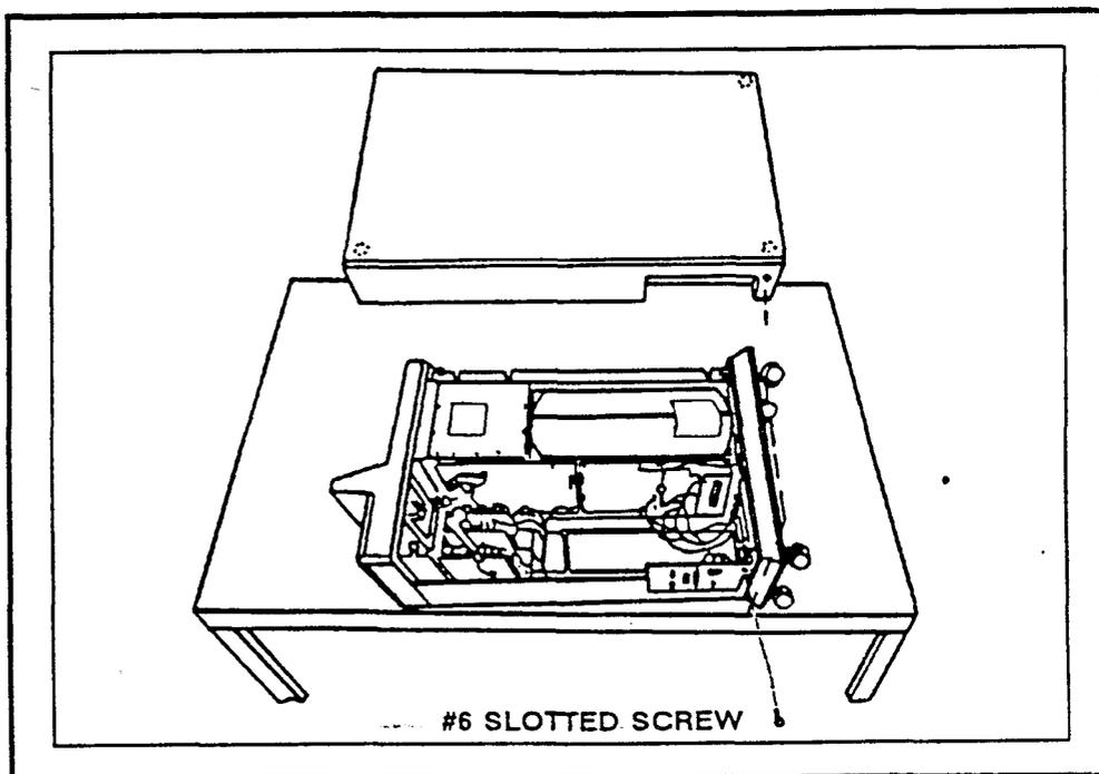
Figure 5-4. Side Cover Removal
