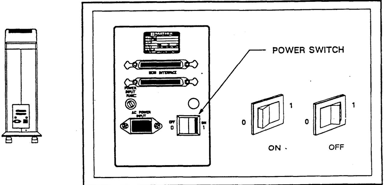
Figure 3-1. POWER Switch Location
