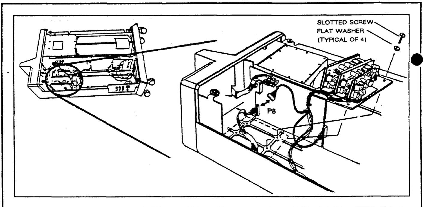
Figure 5-5. Low Voltage Power Supply Removal
