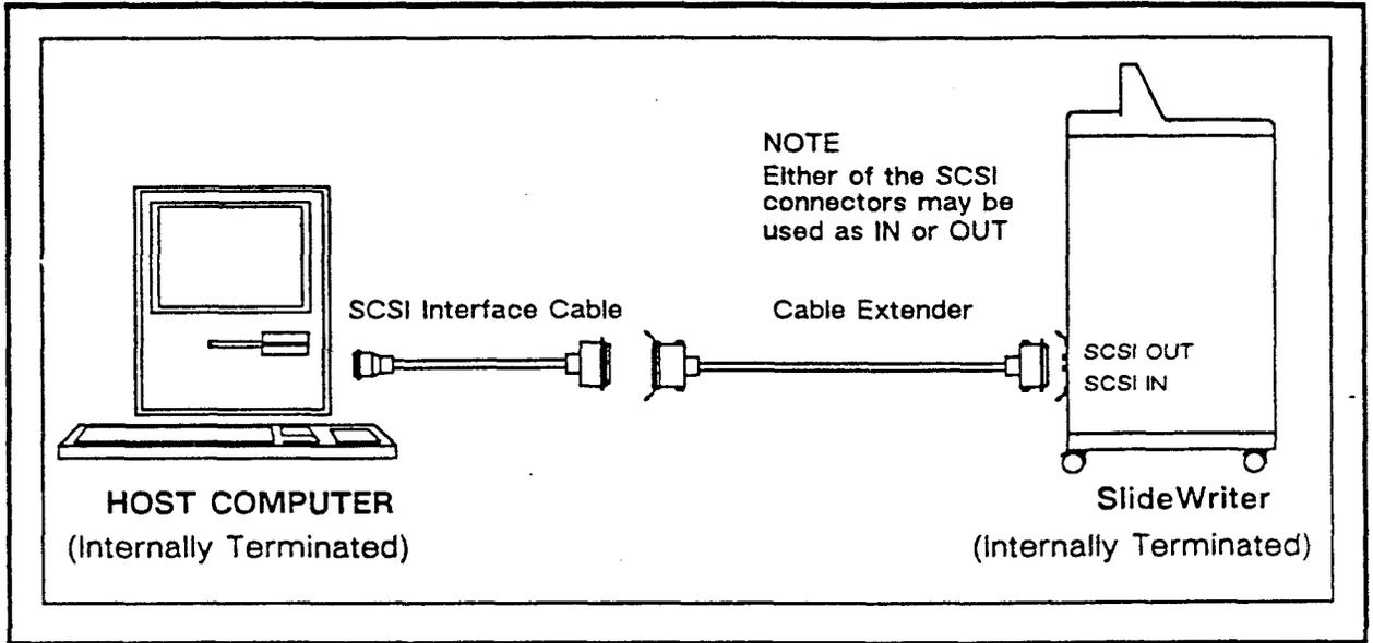
Figure 2-4. Single Device Setup, Both Host and SlideWriter Terminated Internally
