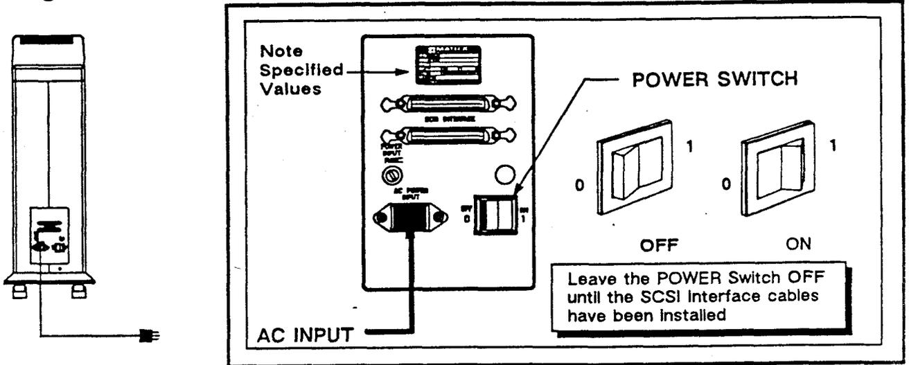
Figure 2-1. POWER Switch and Connector Location
