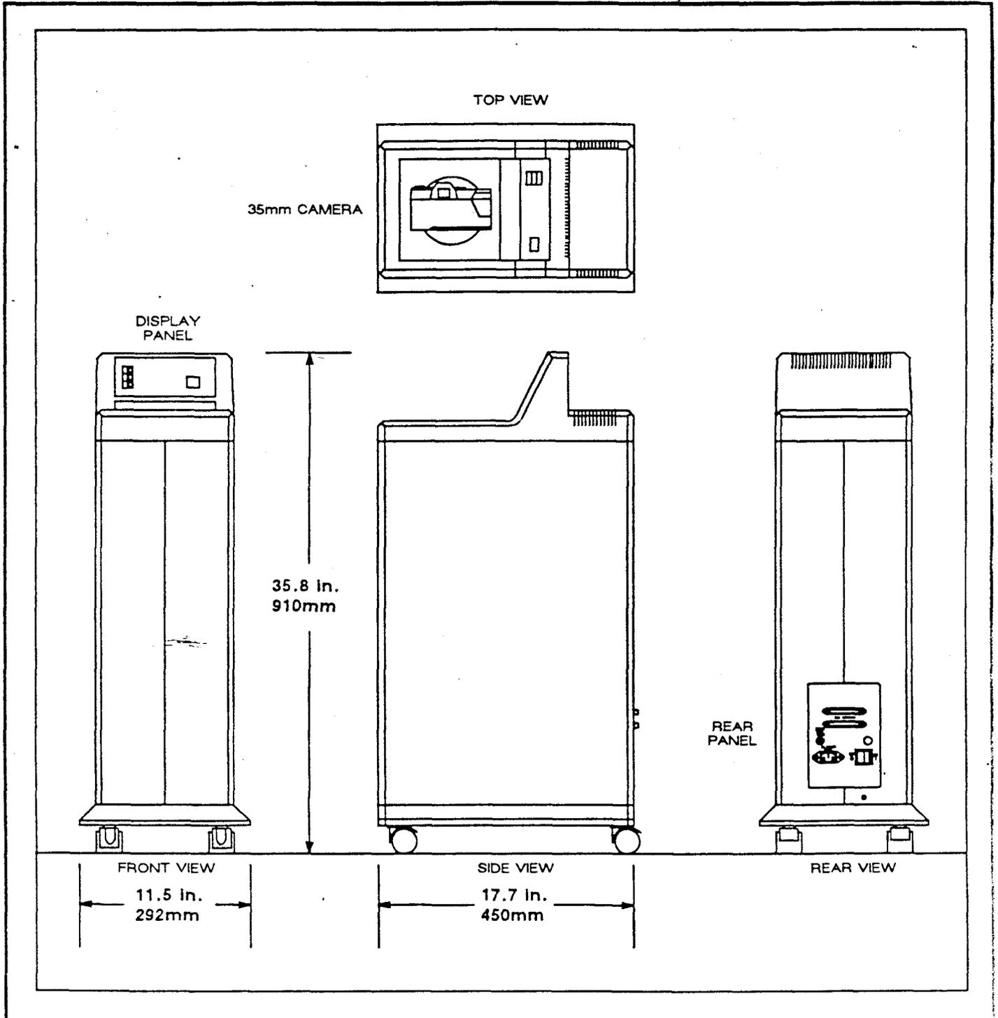
Figure 1-2. SlideWriter Dimensions and External Features
