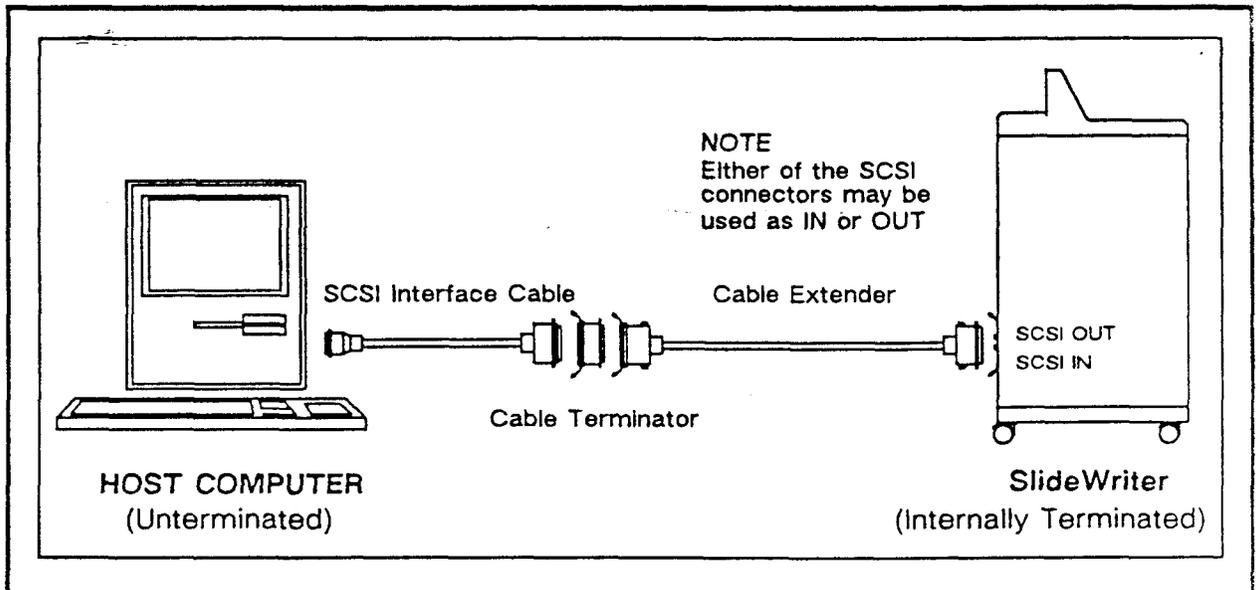
Figure 2-3. Single Device Setup, Unterminated Macintosh Plus with Cable Extender
