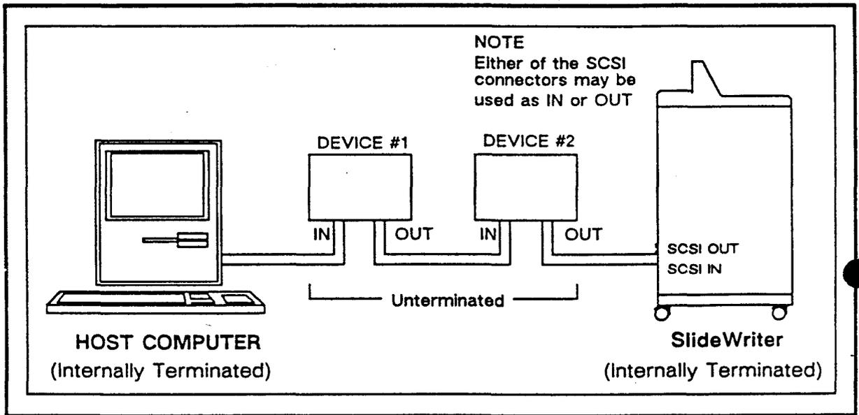
Figure 2-5. Recommended Multiple Device Setup, Both Host and SlideWriter Terminated Internally
