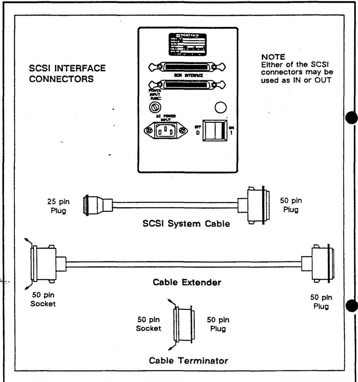
Figure 2-2. SCSI Interface Connectors and Cables
